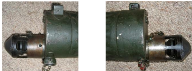
Muzzle attachment, foresight & hose connection, drain plug
